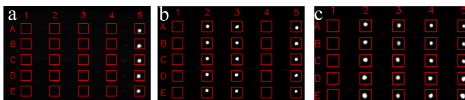
Figure 6. CCD chip images of measurements of (a) SARS-CoV-2 serology-negative sample, (b) sample from a vaccinated individual, and (c) sample from a COVID-19 reconvalescent person (column 1: negative control, column 2: RBD, column 3: S1 protein, column 4: N protein, column 5: positive control, rows A–E represent replicates of the same spot).
