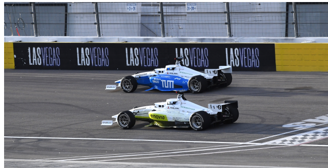
Figure 1. Dallara AV-21: Full-scale prototype of TUM Autonomous Motorsports (back) running the proposed planning algorithm at the LVMS and overtaking a dynamic obstacle.
