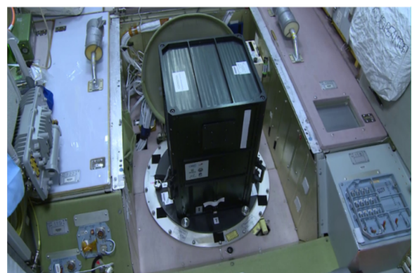
Figure 2. Flight model installed inside the ISS on the UV transparent window of the Zvezda module.
