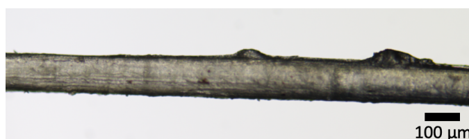
Figure S41: Spun iPP-5 fiber. Conditions: 1500 rpm extrusion speed, 55 rpm KPG stirrer spinning speed, 20 cm distance nozzle – cone, 1 mm manufactured spinning nozzle.
