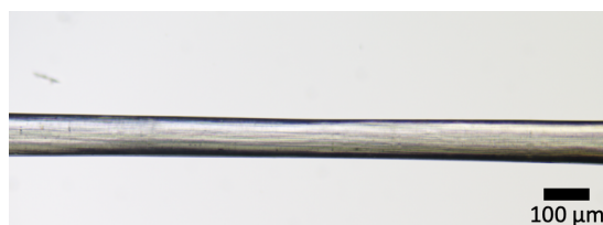
Figure S29: Spun iPP-2 fiber. Conditions: 1400 rpm extrusion speed, 100 rpm KPG stirrer spinning speed, 20 cm distance nozzle – cone, 1 mm manufactured spinning nozzle.
