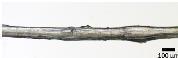
Figure S30: Inhomogeneous spun iPP-3 fiber. Conditions: 1400 rpm extrusion speed, 70 rpm KPG stirrer spinning speed, 20 cm distance nozzle – cone, 1 mm manufactured spinning nozzle.
