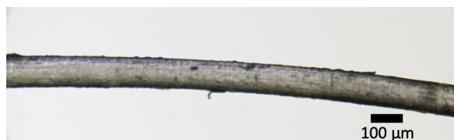
Figure S40: Spun iPP-5 fiber. Conditions: 1500 rpm extrusion speed, 55 rpm KPG stirrer spinning speed, 20 cm distance nozzle – cone, 1 mm manufactured spinning nozzle.
