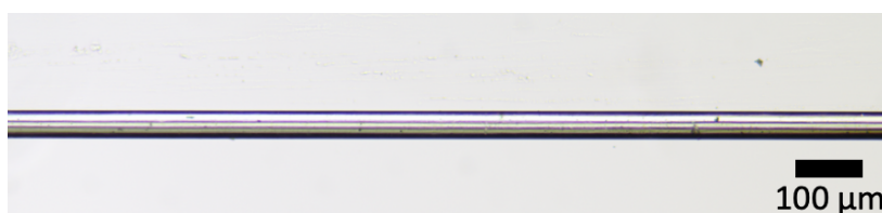
Figure S28: Thin fiber of iPP-2 . Conditions: 1400 rpm extrusion speed, 150 rpm KPG stirrer spinning speed, 30 cm distance nozzle – cone, 1 mm manufactured spinning nozzle.
