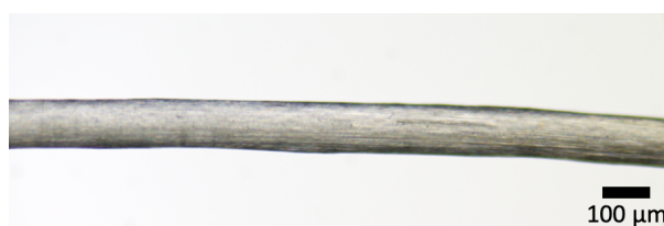
Figure S42: Spun composite fiber. Conditions: 1500 rpm extrusion speed, 78 rpm KPG stirrer spinning speed, 23 cm distance nozzle – cone, 1 mm manufactured spinning nozzle.
