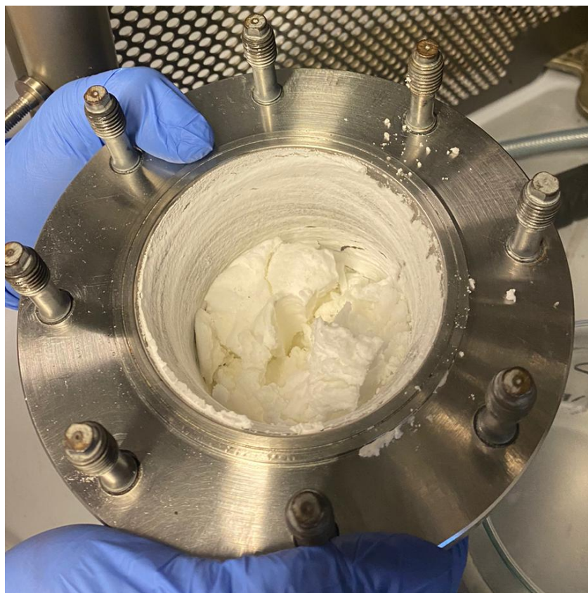
Figure S1. Precipitated sPP in the autoclave after polymerization with I (see entry 1-3, Table 1).
