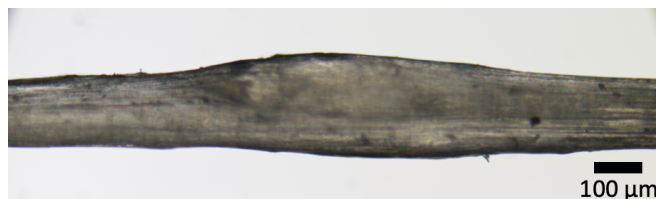
Figure S35: Spun iPP-4 fiber. Conditions: 1500 rpm extrusion speed, 55 rpm KPG stirrer spinning speed, 18 cm distance nozzle – cone, 2 mm extrusion nozzle.
