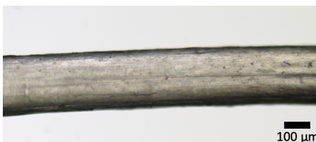
Figure S39: Spun iPP-5 fiber. Conditions: 1500 rpm extrusion speed, 55 rpm KPG stirrer spinning speed, 23 cm distance nozzle – cone, 2 mm extrusion nozzle.
