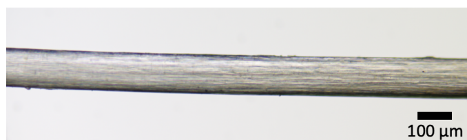
Figure S34: Spun iPP-4 fiber. Conditions: 1500 rpm extrusion speed, 55 rpm KPG stirrer spinning speed, 18 cm distance nozzle – cone, 2 mm extrusion nozzle.
