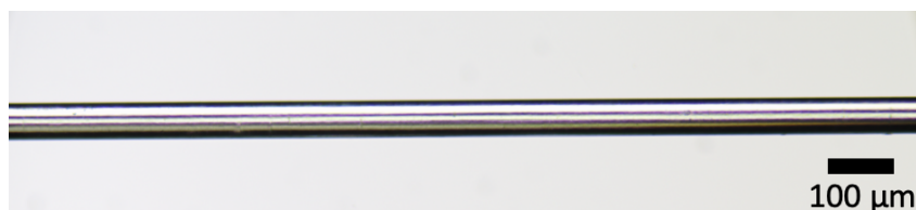
Figure S26: Thin fiber of iPP-1 . Conditions: 1500 rpm extrusion speed, 350 rpm KPG stirrer spinning speed, 140 cm distance nozzle – cone, 1 mm manufactured spinning nozzle.
