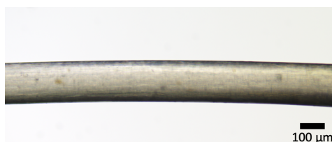
Figure S31: Spun iPP-3 fiber. Conditions: 1400 rpm extrusion speed, 78 rpm KPG stirrer spinning speed, 33 cm distance nozzle – cone, 2 mm extrusion nozzle.
