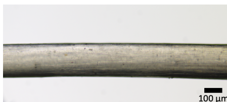
Figure S38: Spun iPP-5 fiber. Conditions: 1500 rpm extrusion speed, 60 rpm KPG stirrer spinning speed, 25 cm distance nozzle – cone, 2 mm extrusion nozzle.
