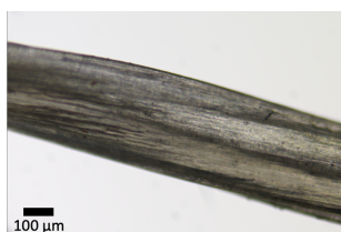
Figure S36: Spun iPP-4 fiber. Conditions: 1500 rpm extrusion speed, 120 rpm KPG stirrer spinning speed, 28 cm distance nozzle – cone, 2 mm extrusion nozzle.
