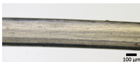
Figure S32: Spun iPP-3 fiber. Conditions: 1400 rpm extrusion speed, 117 rpm KPG stirrer spinning speed, 37 cm distance nozzle – cone, 2 mm extrusion nozzle.
