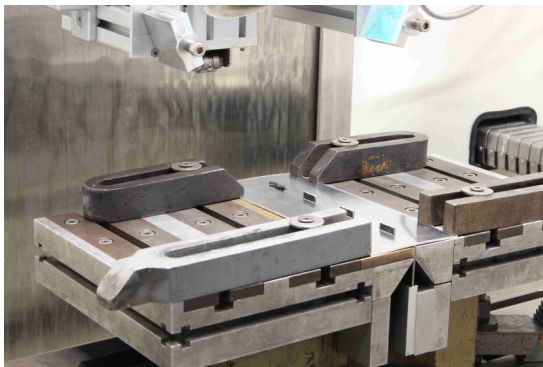
(a) Joining process of a deck panel with four bridges each of 20.0 mm length
