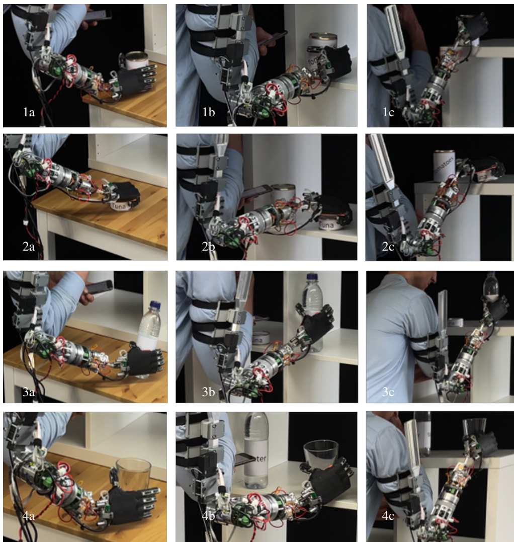
Figure 5.24 Grasping validation for different grasping poses using the SoftHand Pro 2
