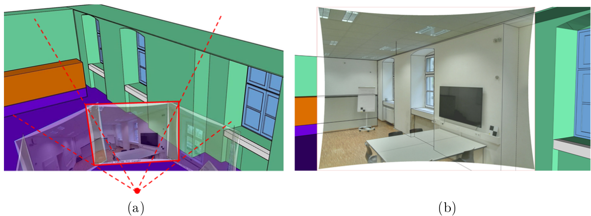
Figure 3.1: Image sequence within a BIM environment: a) image orientation with respect to a BIM's reference system, b) image overlaid with BIM
