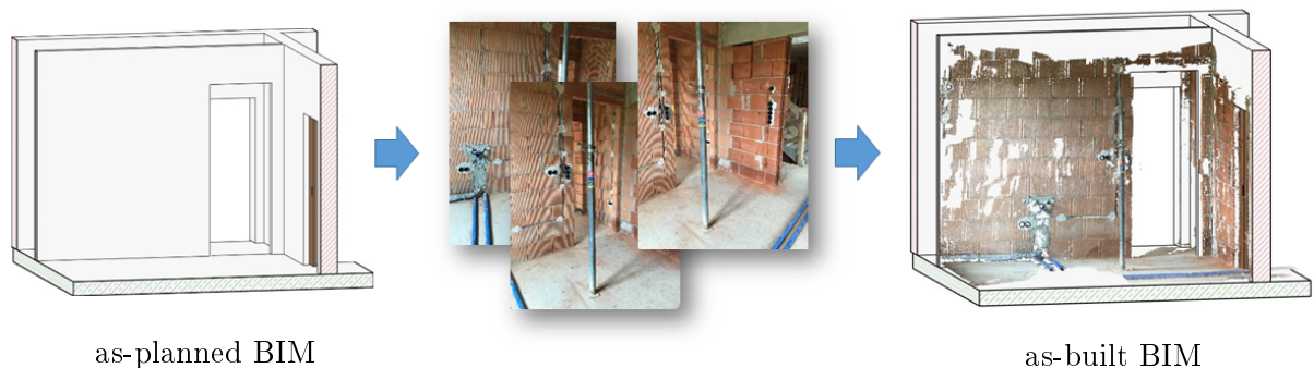
Figure 1.1: BIM transition from as-planned (left) to as-built (right) using image data and generated 3D point clouds
