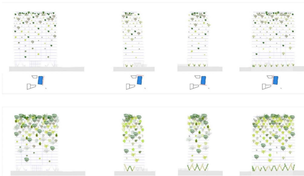
Figure 3. Expected plant growth and facade cover by the architects in the first year ( top ) and 10–15 years after completion ( bottom ) and each façade orientation; east, north, south and west (from left to right). The façade orientation is also marked with a red line in the plan in the middle of the figure according to each façade face. The tour de la biodiversité is the blue marked building in the plan. (Maison Edouard Francois 2016).
