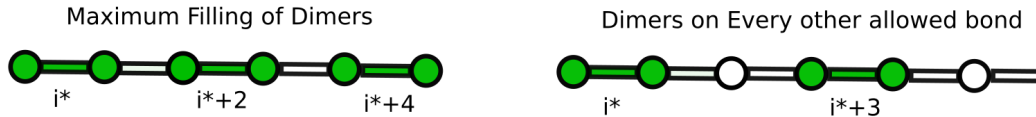
Figure 2.6: Left: A lattice fully filled with fermions hosts one dimer every two links. This shows that half-filling is the maximum possible filling for the effective dimer model. Right: A Mott state with one dimer every three links, corresponding to a density of fermions \rho_F = 2/3 .
