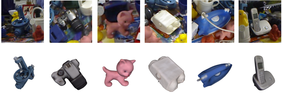
Figure 3.3: Examples of the domain gap between real and synthetic data. The top row illustrates patches with objects taken from the real test images. The bottom row illustrates rendered CAD models of the respective objects.
