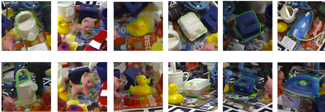
Figure 3.2: Examples of precise and imprecise ground truth pose labels. Green line shows the outline of the object rendered on the image in its ground truth pose. The top row illustrates perfect alignment between the object in the image and the rendered object. The bottom row, on the other hand, demonstrates imprecise alignment which indicates imprecise ground truth poses. All poses are real ground truth annotations from Linemod [5]
