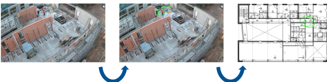
Figure 2: Image processing method using object detection to process the location of workers
