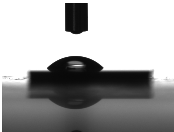
Figure A.12.: SWCA measurements of acid cleaned diamond show a rather hydrophilic surface of 46 \pm 0.9 degrees.
