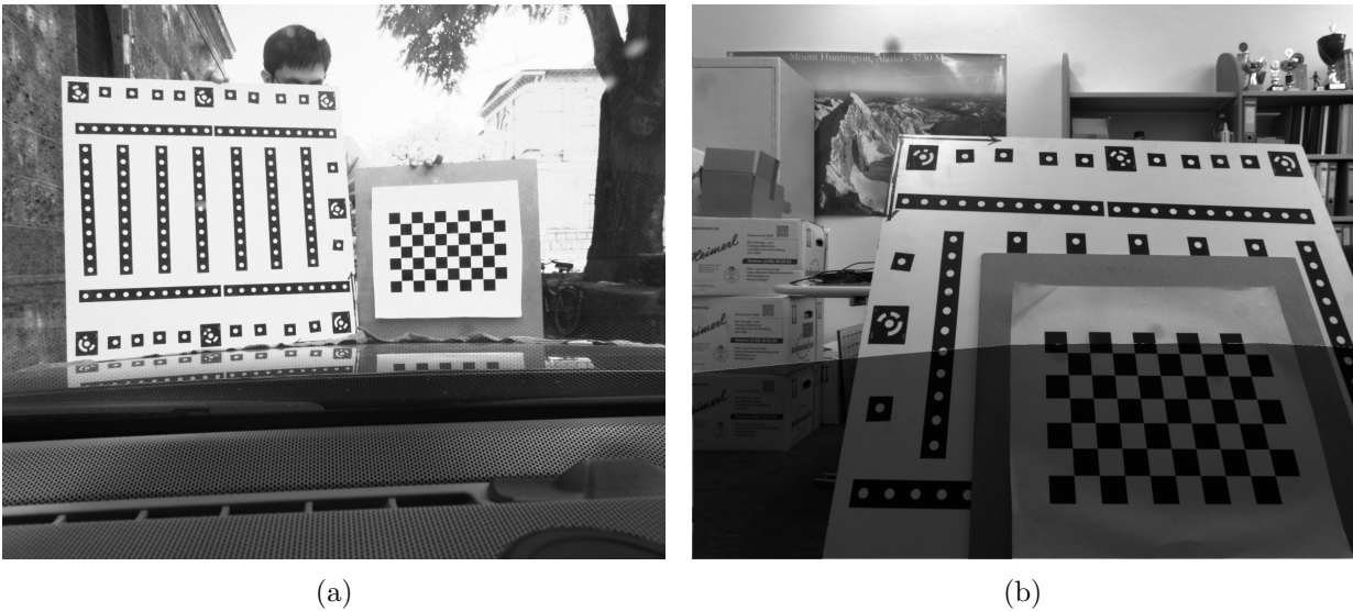
Figure 4.3: Example images from the Stereo image dataset showing the virtual 3d test field. a) With windshield setup: Cameras in the car, b) without windshield setup: Cameras in the lab. The bonnet area is masked (half-transparent dark overlay) so that reference point positions are comparable in both setups.
