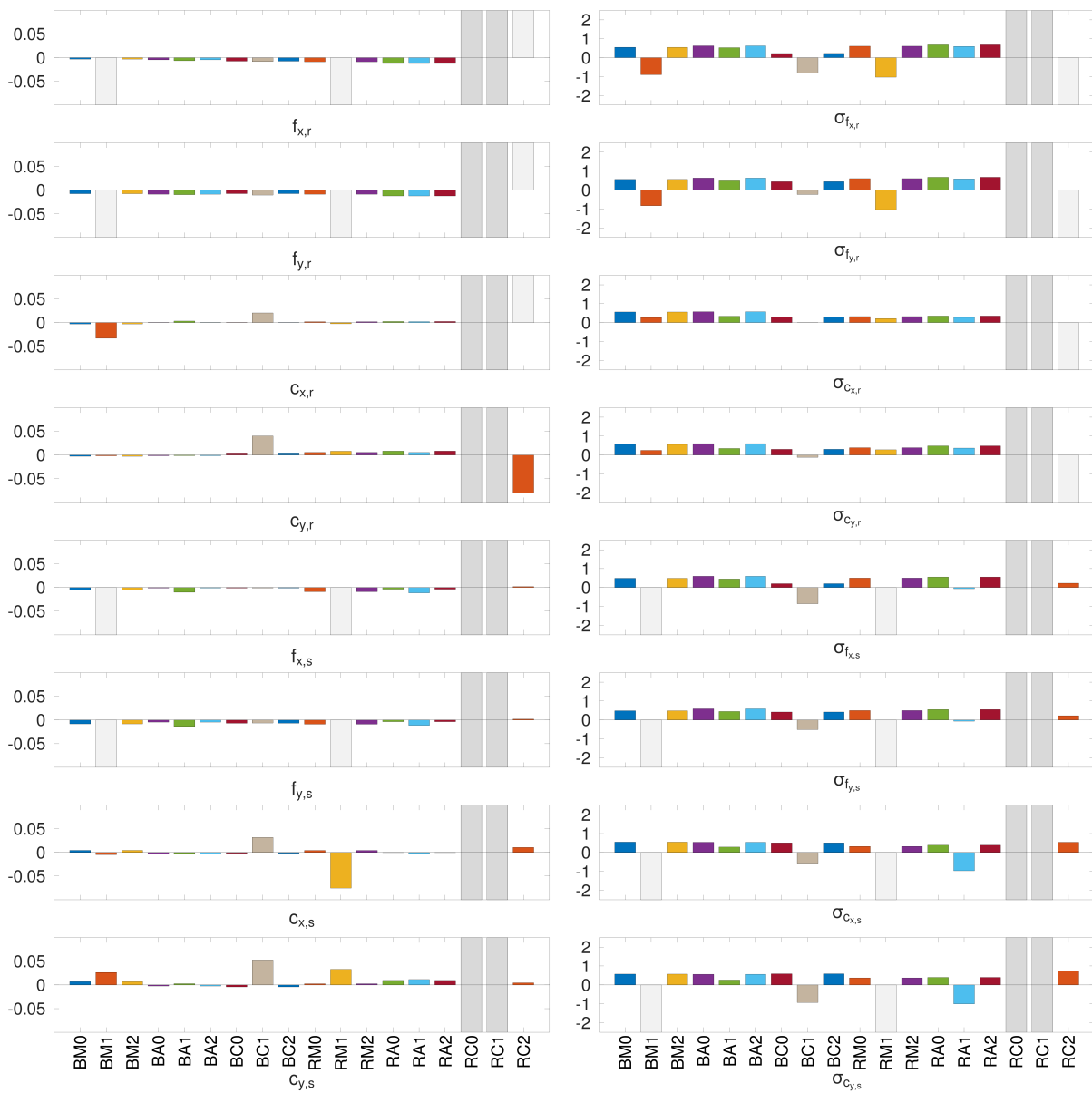
Figure 8.3: Relative deviations of focal length and principal point parameters between the with and without windshield setup. Reference and slave camera, all feature types, all stereo constraints and two camera models shown. Descriptions of the abbreviations see Figure 8.1. Vertical axis unit-free, invalid deviations in medium gray, off-limit deviations in light gray.
