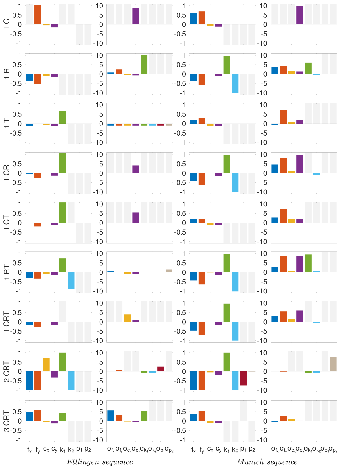
Figure 8.11: Relative deviations of the estimated interior orientation parameter values and standard deviations between camera calibration with traffic signs and reference calibration. The vertical axis is unit-free due to relative deviations, off-limit deviations are colored in light gray. Descriptions of the abbreviations see Table 8.4.
