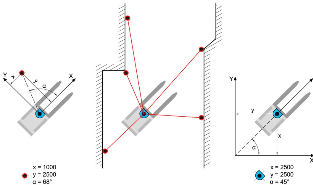
**Figure 2.** Basic sketch of the determination of the relative position between the reference mark and the vehicle (left) and the absolute position in the coordinate system (right) (Adapted after SICK AG, in [5]).
