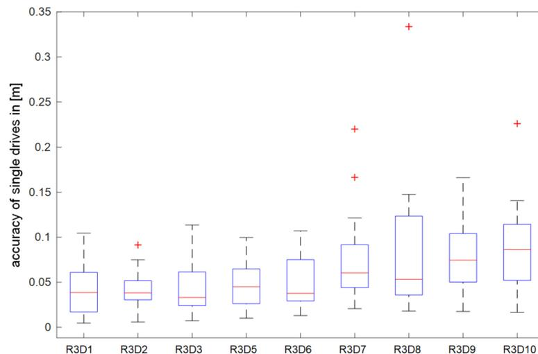
**Figure 9.** The box plots show the deviations of the closest neighbors (accuracy) for each single drive from run 3 in the route section. (+—maximum deviation).
