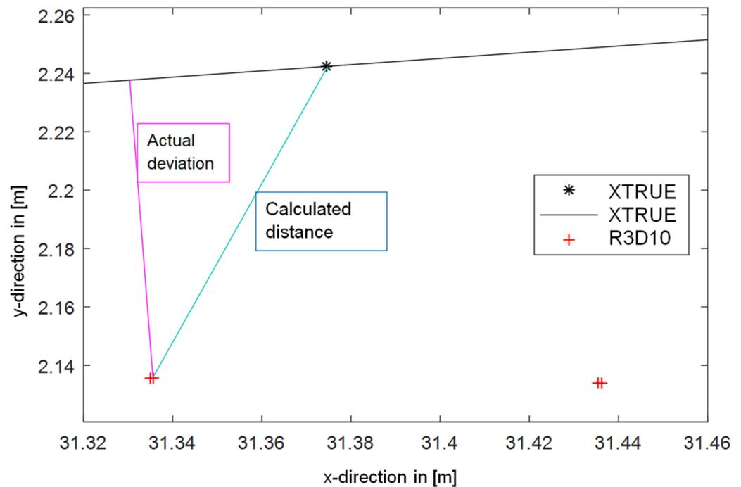
**Figure 8.** With the 1NN method, the Euclidean calculated distance could only approximate the true distance. Herein, the calculated distance of a point of the trajectory R3D10 is, for example, greater than the actual deviation.
