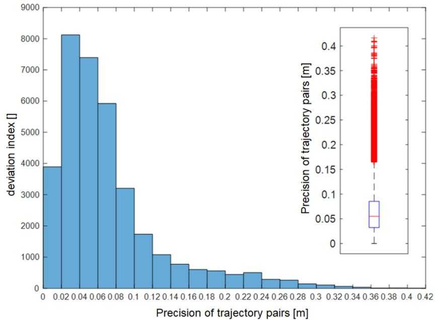
**Figure 12.** The histogram shows the statistical relationship between the precision of the nine drives taken from run 3 in the route section.
