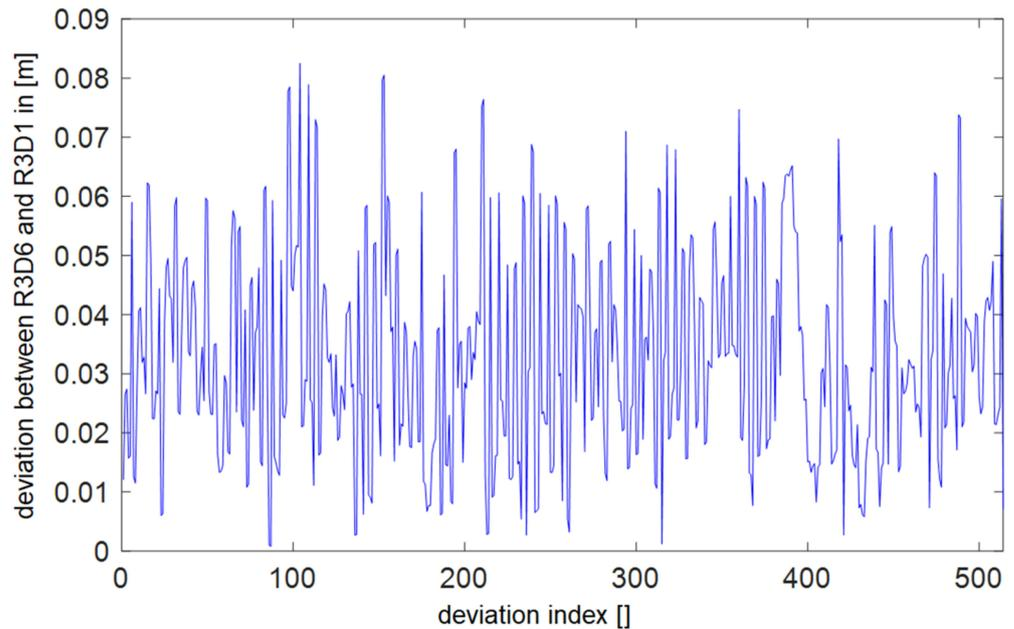
Figure 10. The precision calculated using the 1NN method for the drives R3D6 and R3D1. The precision was between 0.0008 and 0.0825 m.
