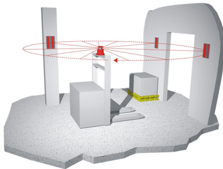
**Figure 1.** The rotating laser scanner is mounted on the vehicle and measures the reference marks on pillars and walls. Reprinted/adapted with permission from Ref. [21]. 2018, Götting KG.
