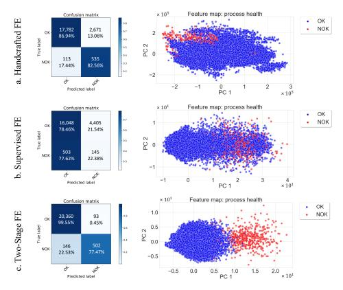
**Figure 8.** Comparison of the handcrafted (**a**), supervised (**b**), and the proposed method (**c**) trained feature extractors: the top row shows the confusion matrices obtained by the MLP classification, and the bottom row shows the 2D visualization of the FEs' feature spaces.
