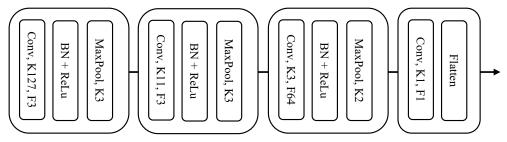
**Figure 3.** Architecture of the deep feature extractor  $f_{\theta}$ . MaxPool: maxpooling layer; Conv: 1D convolutional layer; BN: batch-normalization; K: kernel size; F: filter channels
