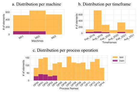
**Figure 4.** Distribution of the training and test datasets per machine, timeframe, and machining process. To reflect the challenges of industrial practice, a limited amount of data is included in the training set (violet) and unseen data from different machines, time periods and process operations is included in the test set (orange).
