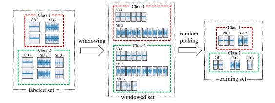
**Figure 1.** Mixture-based data selection method used in a 2-way and 5-shot FSL for single-axis vibration signals (C = 1). SB: subclass
