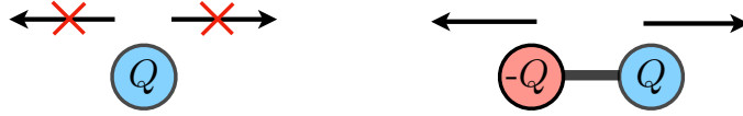
Figure 2.5: Fractons in dipole-conserving systems. In systems with dipole-conservation, single charges are immobile and correspond to fractons. In contrast, dipole objects composed of two fractons can move freely.
