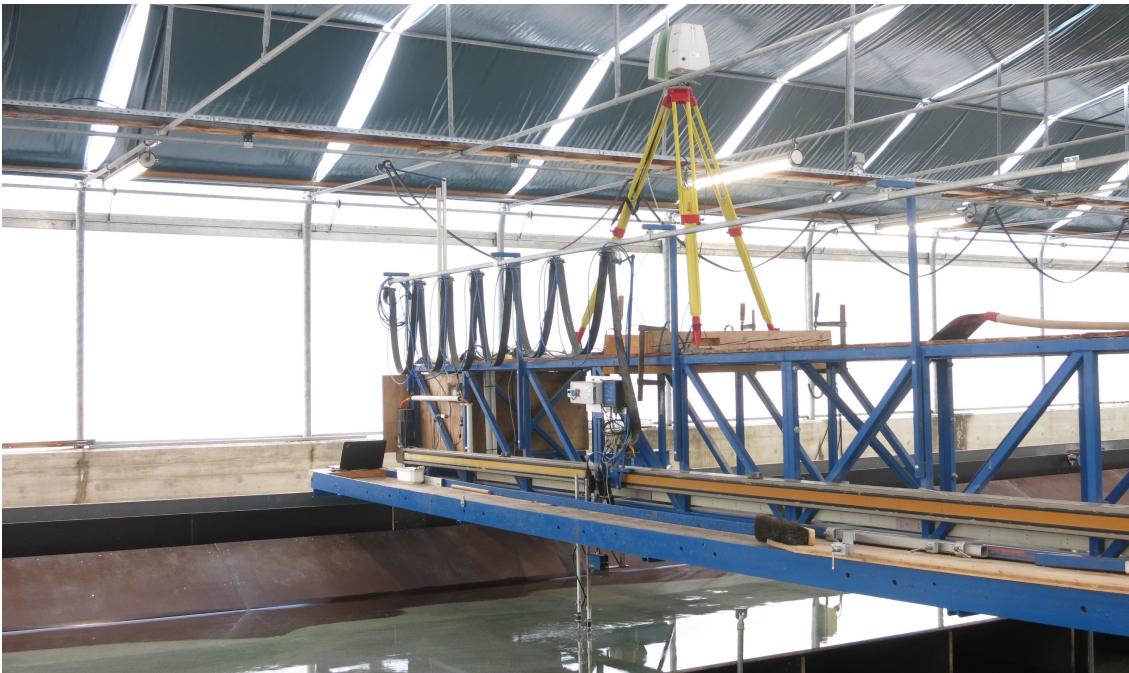
Figure 19: Measuring cart with laser scanner and ADV probes during operation
