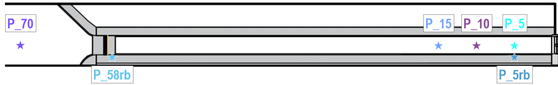
Figure 16: Location and labeling of pressure sensors for water level measurement in the river reservoir
