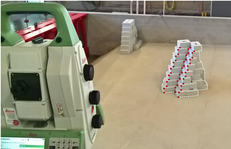
Figure 4. Experimental setup of a reference object to provide object control points (highlighted in red). The measurements were carried out using a Leica ScanStation C10 even though in this sample image another instrument is shown.
