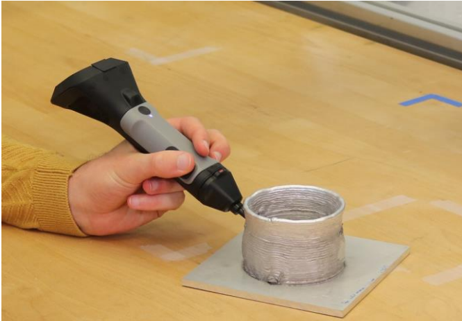
Figure 4: Spatially annotating the defects in the sample part using the VR tracker by Wandelbots™. The obtained coordinates must be transferred from the tracker coordinate system to the component coordinate system using coordinate transformations.
