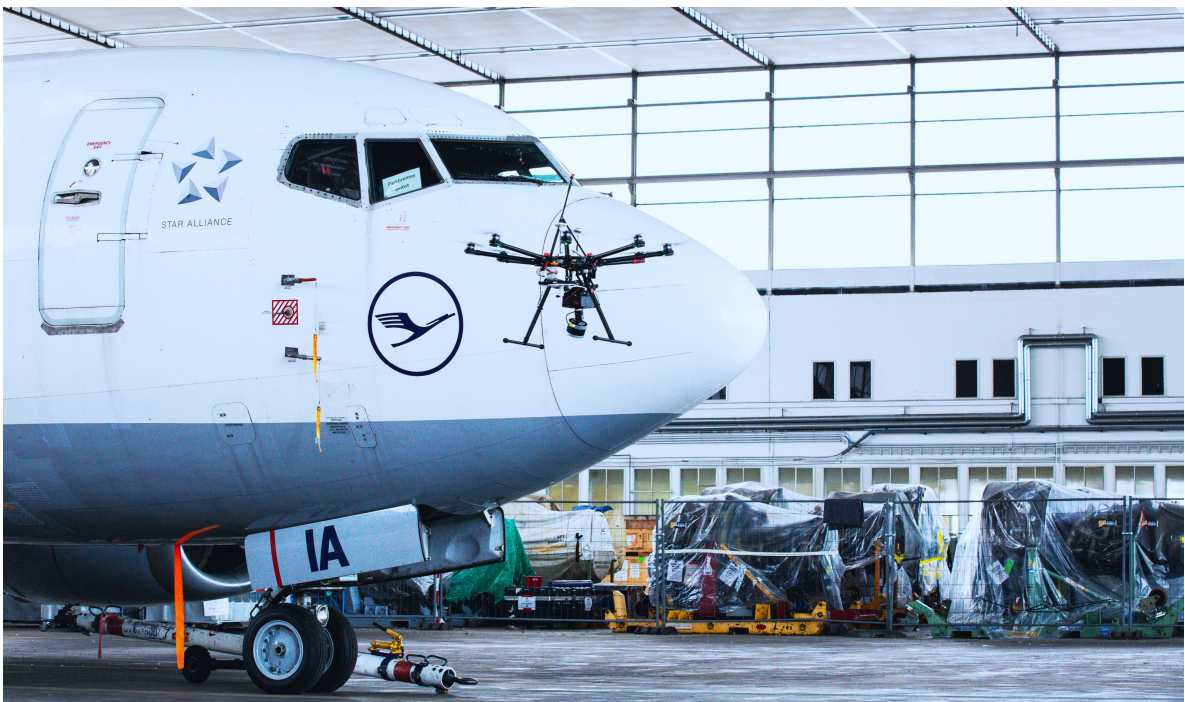
Figure 1.1: Airplane autonomous inspection using UAVs. An example where real-time motion estimates and mapping are needed simultaneously for navigation. In such applications, high-accuracy GPS/INS systems are impractical due to the weight, cost, and external magnetic perturbations. GPS signals are also unreliable underneath the structures of the hangar. Camera-based localization systems, on the other hand, provide poor performance and this is mainly due to the texture-less surfaces and far-field view. The UAV's navigation stack requires 6D motion estimation. The estimation latency is critical in such applications as the robot experiences a very fast motion behavior.
