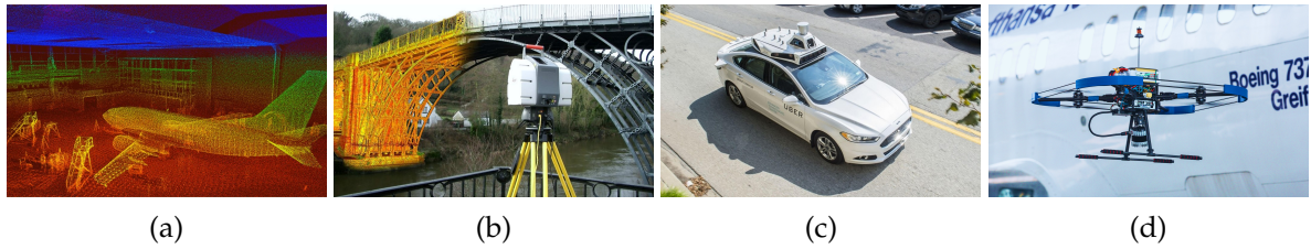
Figure 1.2: (a) A map of an indoor area. (b) A Leica scanner attached to a tripod. (c) A laser scanner and industry grade GPS/INS mounted on an autonomous car. The car is equipped with multiple GPS/INS systems and uses the Differential GPS (DGPS) to provide precise motion estimates. (d) Autonomous drone for airplane inspection and mapping. In such application, high-accuracy GPS/INS systems are impractical due to the weight and cost. GPS signals are also unreliable inside the hangar or below structures of the buildings. The latency of the estimation is critical for real-time navigation.
