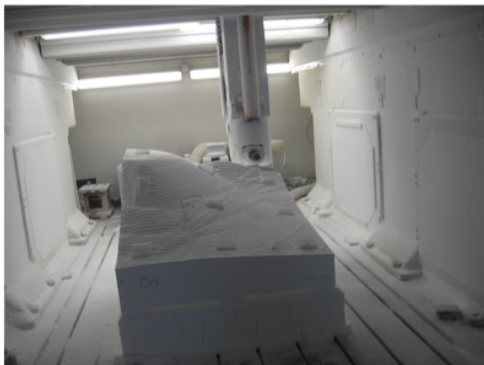
Figure 7: A complex sub-part cut by CNC machine.
