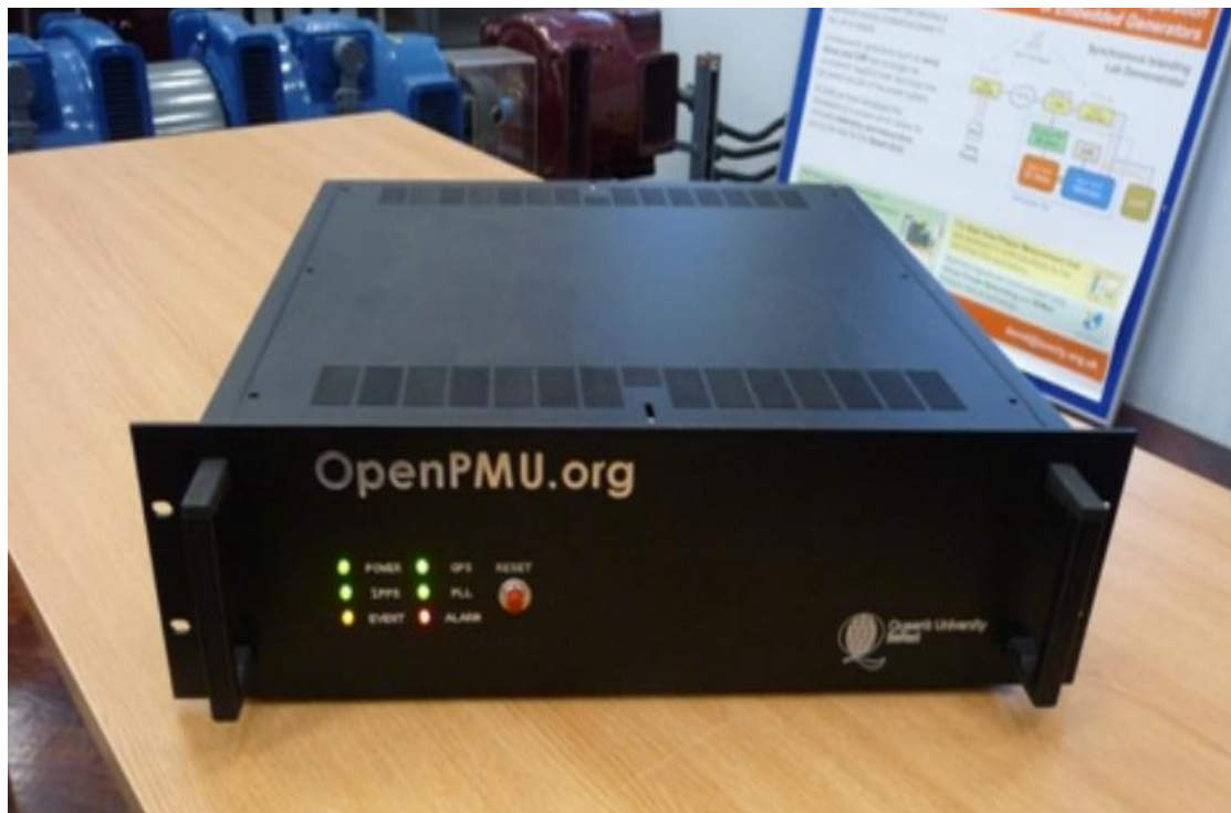
Figure 2. OpenPMU V1. Photo: Credits to National Instrument [19].
