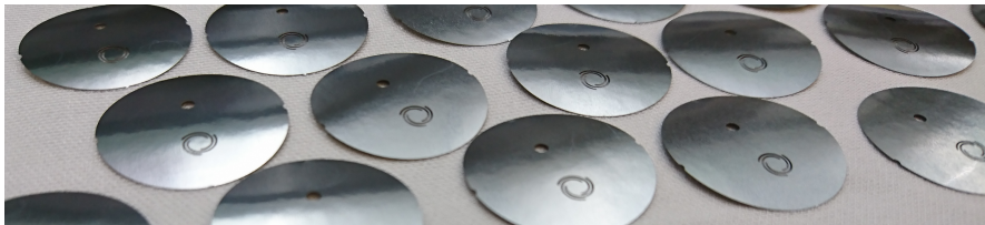
Figure 6: Photograph of cold-rolled, photochemically machined titanium foils with passive check valve structures. As a result of residual stresses caused by coiling of the sheet material prior to PCM, the 50\ \mu\text{m} thick foils exhibit a noticeable curvature.
