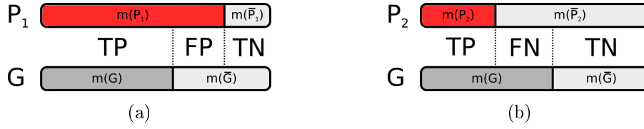
Figure 5.4: Stacked bar charts illustrating the concept of the fuzzy confusion matrix. (a) Example of a false positive caused by an overestimation of A . (b) Example of a false negative caused by an underestimation of A . True positives and true negatives correspond to the minimum overlap of the estimates with the ground truth.
