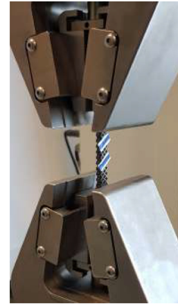
Fig. 7. Experimental setup of a tensile experiment on an octet-truss lattice structure [18].
