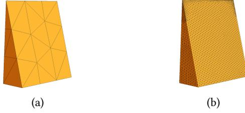
Fig. 4.24: A sharp wedge employed for demonstrating the MFIE's inaccuracy © 2018 IEEE [Kornprobst and Eibert 2018e]. (a) The studied coarse mesh. (b) The refined mesh used for calculating for the EFIE reference solution.
