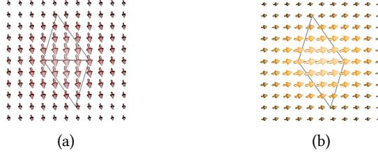
Fig. 3.3: Tangential field (real part) evaluation on a surface placed  $\lambda/20$  over an RWG basis (length  $\lambda/6$ , width  $\lambda/12$ ) for an electric surface current density. (a) Electric field over a planar function. (b) Magnetic field over a planar function.
