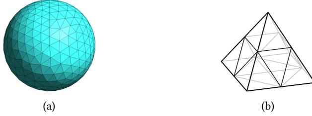
Fig. 4.9: Two models for the analysis of the the WF basis transformation scheme in the RWG-tested MFIE © 2018 IEEE [Kornprobst and Eibert 2018e]. (a) A sphere. (b) A Pyramid.
