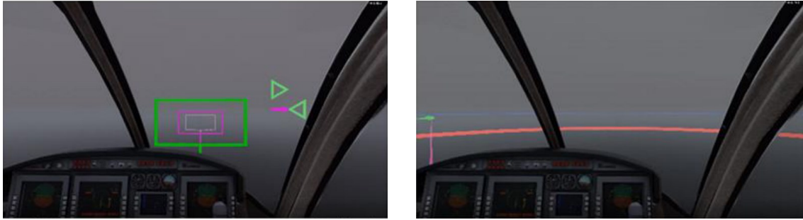
Figure 2-7: HUD presented tunnel in the sky (left) and cueing set (right)
