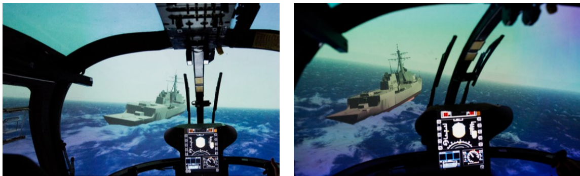
Figure 5-11: Cockpit view - Ship operating in low (left) and high (right) sea states
