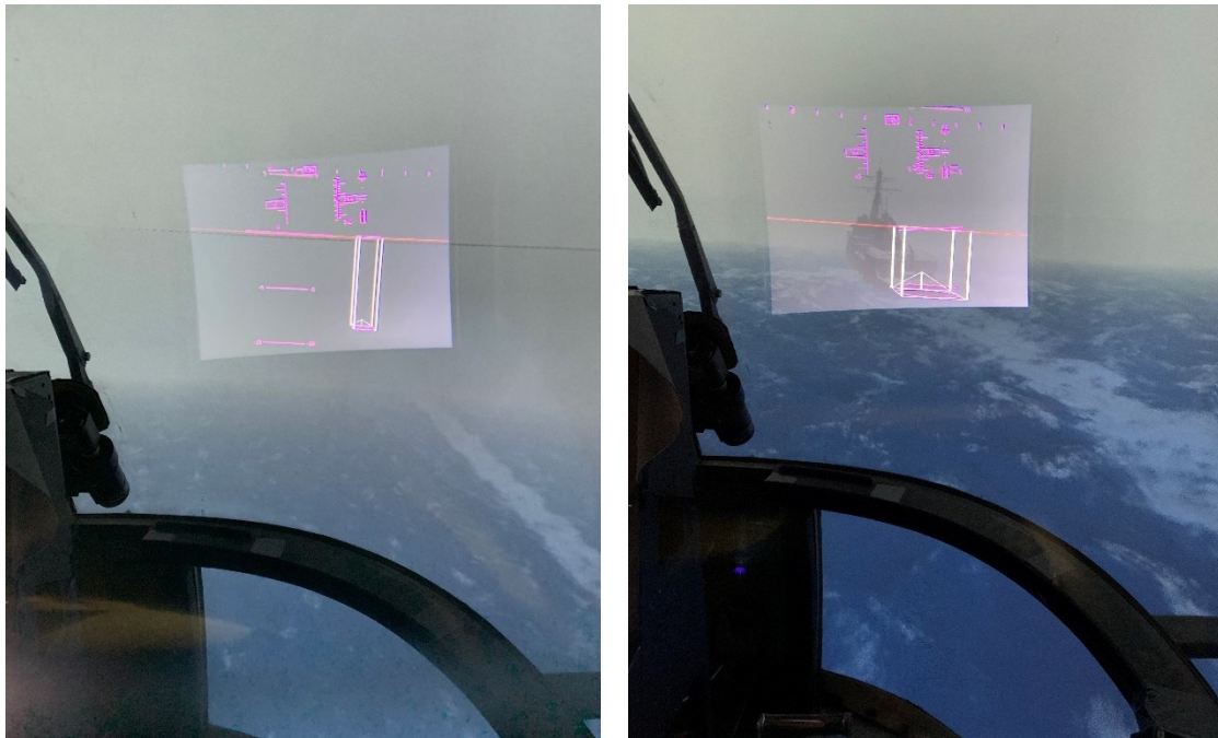
Figure 5-18: HMD symbology as seen from MAP (left) and behind the deck (right)
