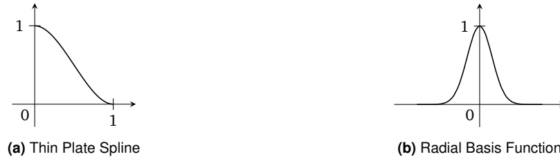
Figure 4.2: Different kernel functions that can be used for modeling a Gaussian Process Implicit Surfaces.
