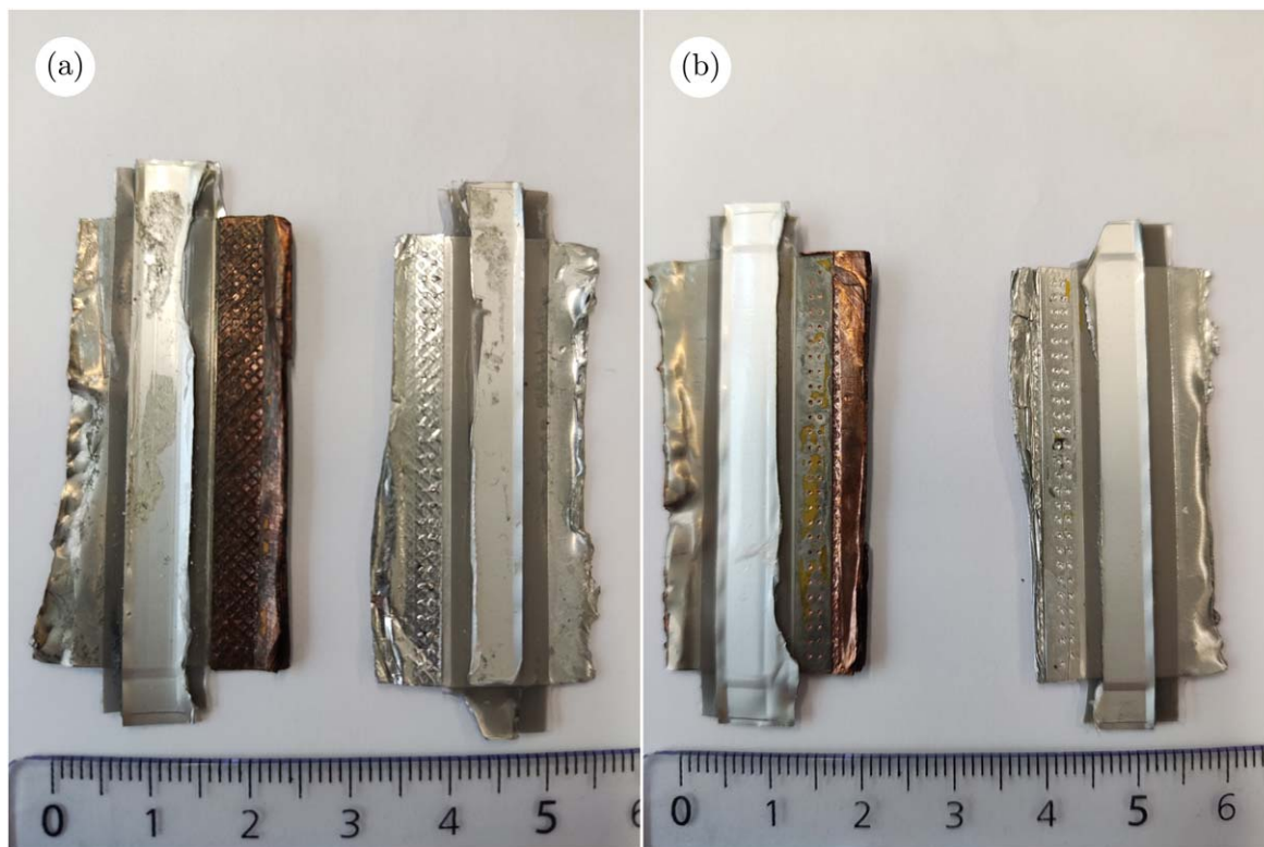
Figure A-2. Embossing on tabs and substrate foil of (a) anode and (b) cathode.
