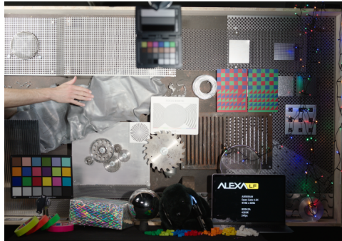
Figure 5.4: Corner Case image which includes colored lights as well as white and colored reflections
