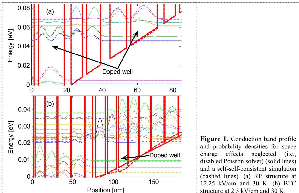
**Figure 1.** Conduction band profile and probability densities for space charge effects neglected (i.e., disabled Poisson solver) (solid lines) and a self-self-consistent simulation (dashed lines). (a) RP structure at 12.25 kV/cm and 30 K. (b) BTC structure at 2.5 kV/cm and 30 K.
