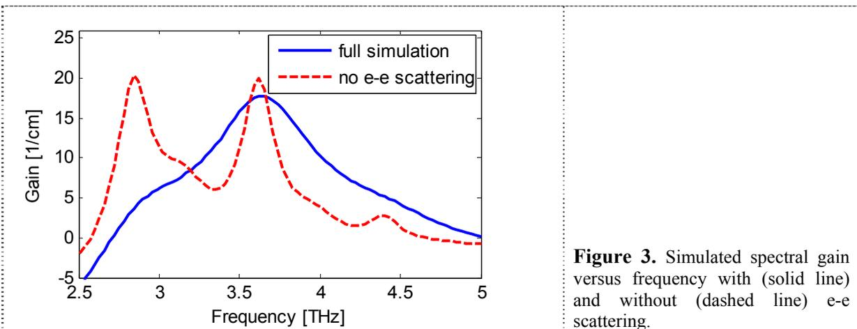
**Figure 3.** Simulated spectral gain versus frequency with (solid line) and without (dashed line) e-e scattering.
