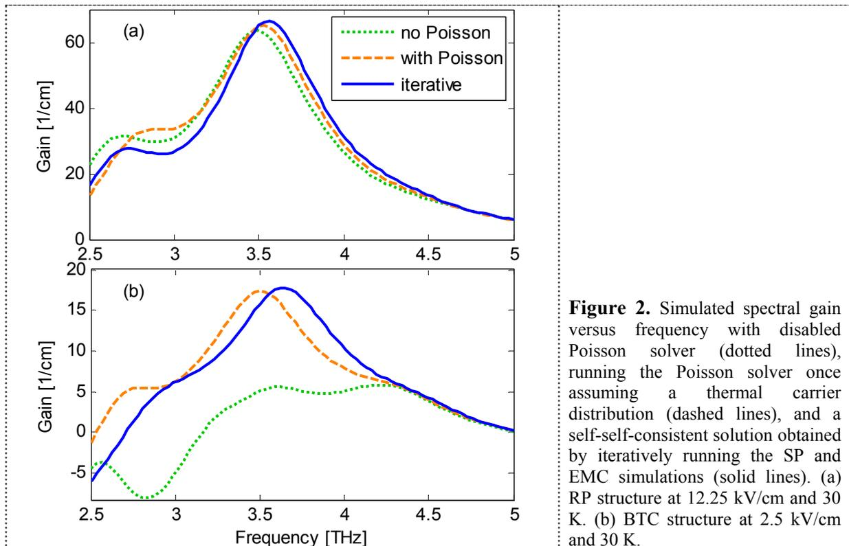
**Figure 2.** Simulated spectral gain versus frequency with disabled Poisson solver (dotted lines), running the Poisson solver once assuming a thermal carrier distribution (dashed lines), and a self-self-consistent solution obtained by iteratively running the SP and EMC simulations (solid lines). (a) RP structure at 12.25 kV/cm and 30 K. (b) BTC structure at 2.5 kV/cm and 30 K.
