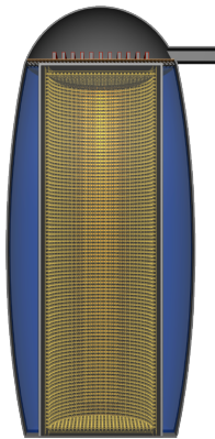
Figure 1. Artistic view of the LENA detector. The diameter of the concrete tank is 32m and the height 100m. The liquid scintillator, coloured in yellow, is monitored by \sim 29,600 optical modules with 12" PMTs mounted on a steel scaffolding. The space between tank and detector cavern is filled with water and serves as a muon veto and additional shielding against external radiation.
