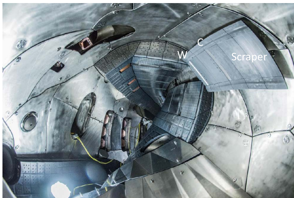
Figure 7. View of a scraper element inside W7-X. The scraper has a W and a Mo/C marker layer close to the Langmuir probe arrays.
