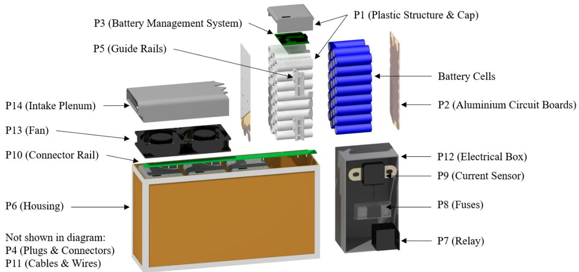
Figure 14: Conchifera electrical vehicle battery system (quadruple variant).
