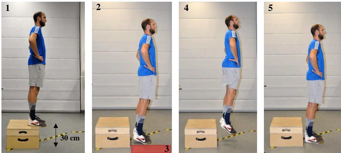
Figure 12 A. Time-course of a drop jump. Participants stand with hands resting in their hips on a 30 cm height (1), followed by a drop (2) onto a ground-integrated force measurement plate (3) and a jump (4) as high as possible. After the jump (5) weight of the participants is measured by the plate in a standing position.
