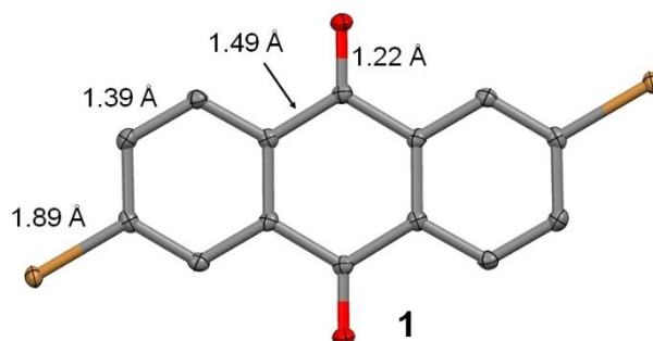
Figure S1. Molecular structure of DBAq. Aromatic hydrogen atoms were omitted for clarity reasons. All ellipsoids are shown at the 50% probability level. Atom colors are grey (C), red (O), brown (Br).
