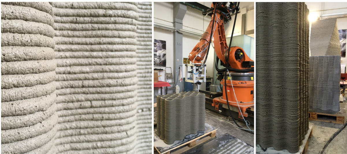
FIGURE 5.2: Extruded lightweight aggregate concrete elements
