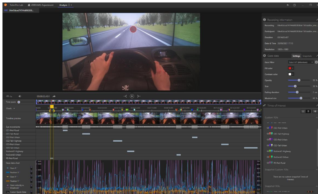
Figure 3.6.: The Time of Interest interface in Tobii Pro Lab V1.162. The 9 grey bars in the bottom half of the picture represent nine events that were logged (6 critical events, 2 non-events and 1 pre-cursor event) (source: own)
