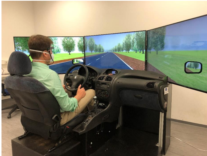
Figure 3.1.: Driving simulator used for stage 1 of the i-DREAMS project at the Chair of Transportation Systems Engineering at TUM (source: own)
