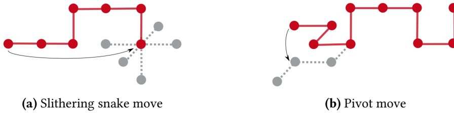
Figure II.5: Global moves. (a) In the slithering snake move an end monomer is removed and reattached in a randomly chosen orientation at the opposite chain end, leading to a reptating motion of the polymer. (b) In the pivot algorithm a monomer is randomly chosen and either the left or the right portion of the chain is rotated in a random way around this monomer.
