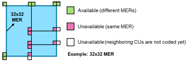
Fig. 10. Illustration of spatial merging candidate insertion with MER.
