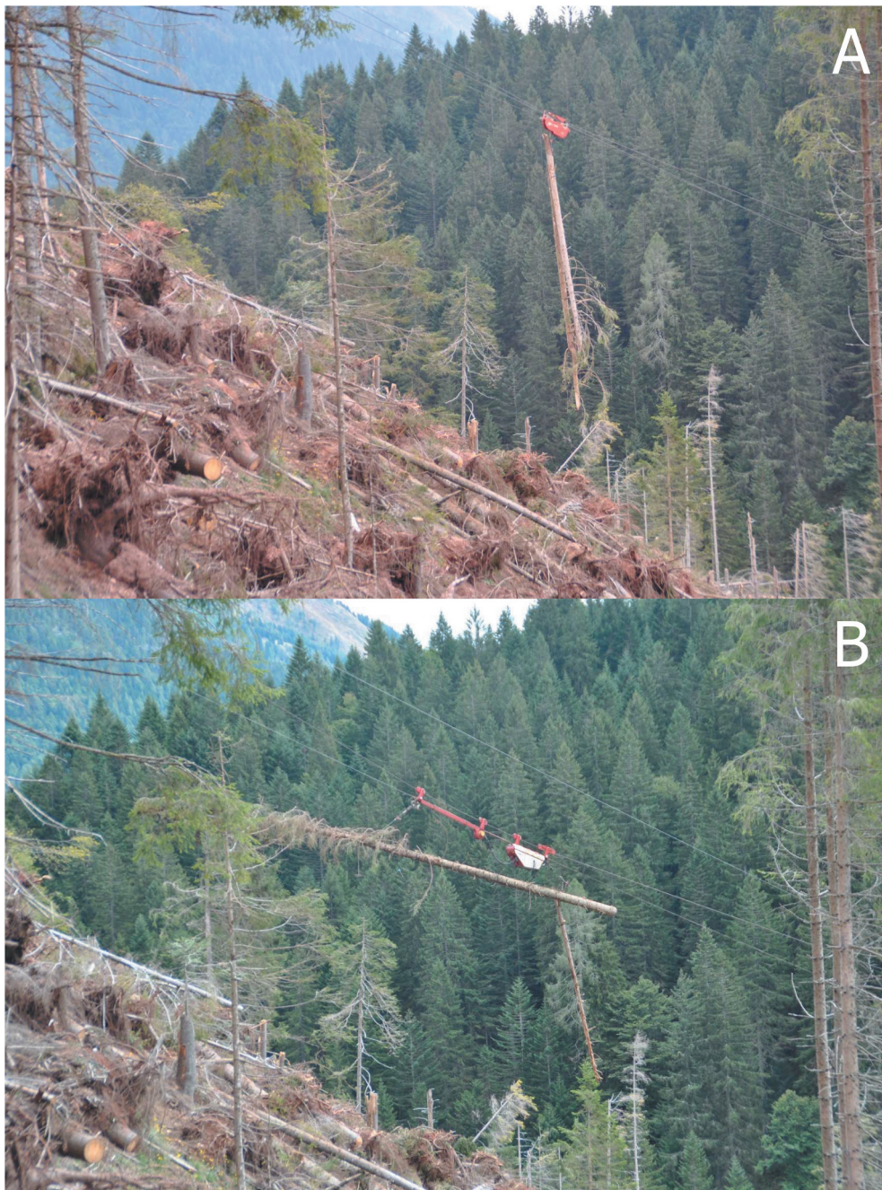
Figure 1. The test set-up running the single (A) and double carriage (B).
