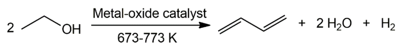
Scheme 1.6 The conversion of ethanol to 1,3-BD in one-step Lebedev process. Adapted with permission from ref. [88]. Copyright (2013) John Wiley and Sons.
