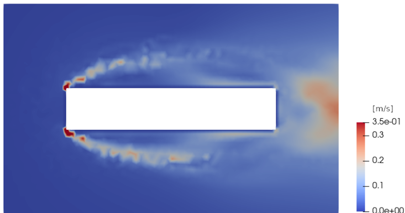
Figure 4.29: Standard deviation of span-wise averaged and time-averaged velocity calculated by MF-NIPC
