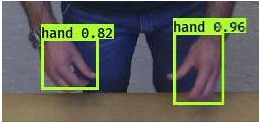
Figure 4.4: Detected hands using the pre-trained YOLO network
