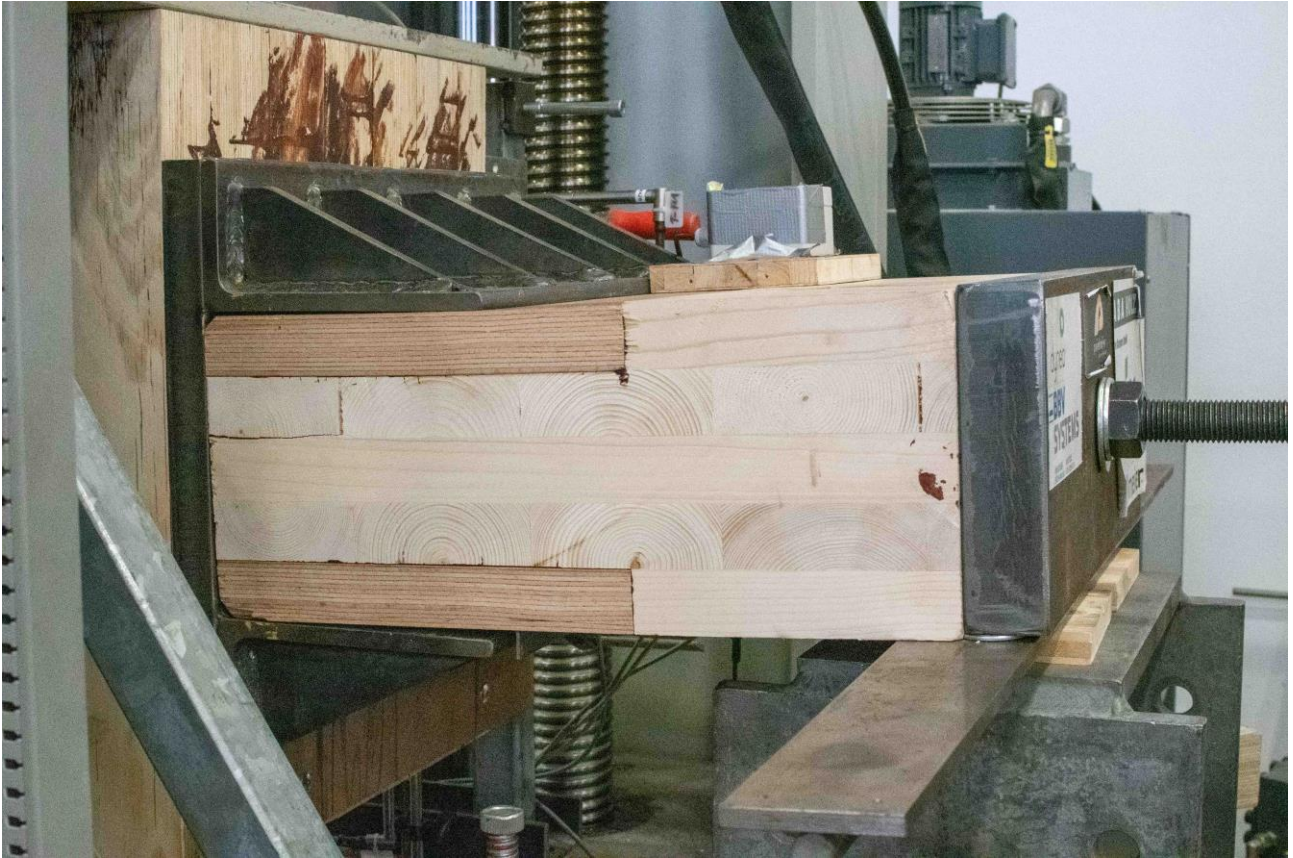
Figure 281 – Rotation of the right horizontal sample during the final cycle of PTT5-3-3, showing the elastic deformation of the horizontal element inside the composed steel plates and the effectiveness of the LVL beech layers in protecting the surface of the horizontal elements during rotation
