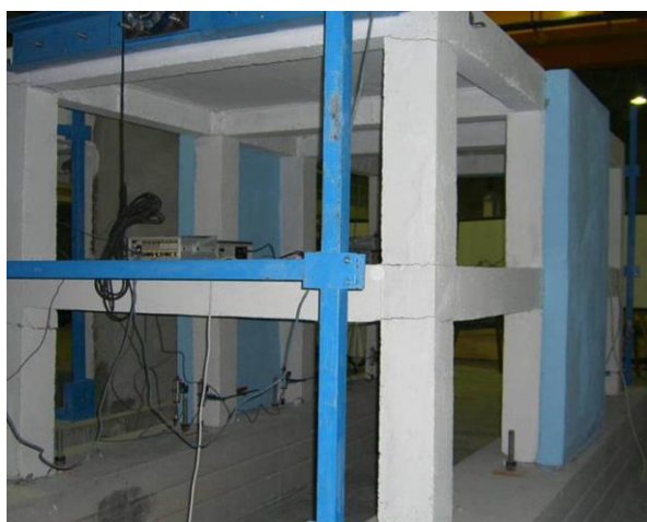
Figure 47 – Photo of the damaged strengthened specimen after the test – Source: [47]
