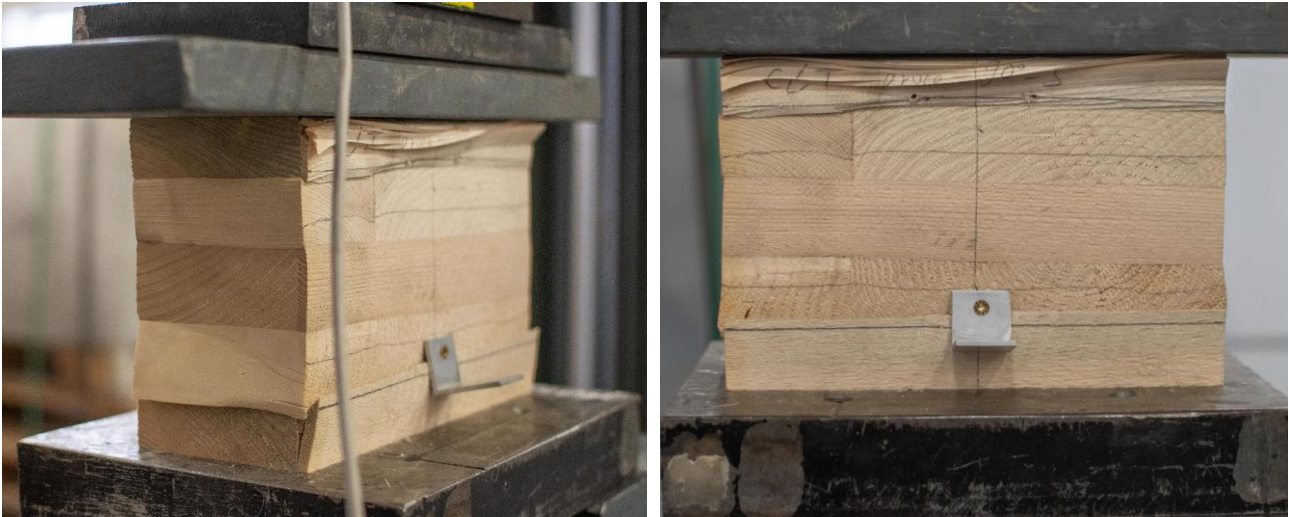
Figure 226 – Highly deformed CLT-piece without transducers – Source: [208]
