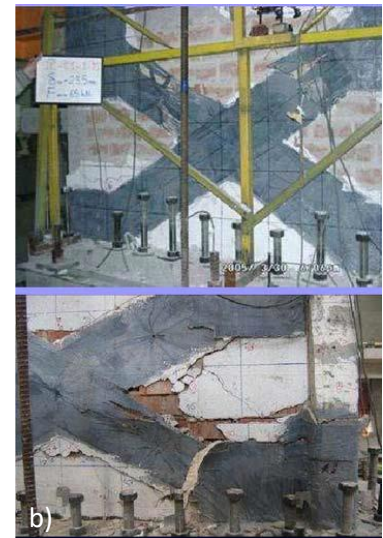
Figure 12 – a) Base shear versus displacement envelopes for bare and infilled frames; b) photos of the damage on infills strengthened with FRP – Source: [41]
