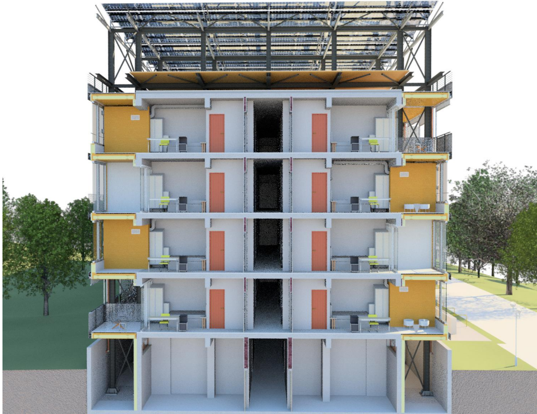
Figure 292 – Axonometric vertical cross-section at the first span of the Athens case study after the application of the Pro-GET-onE strategy – Source: [142]
