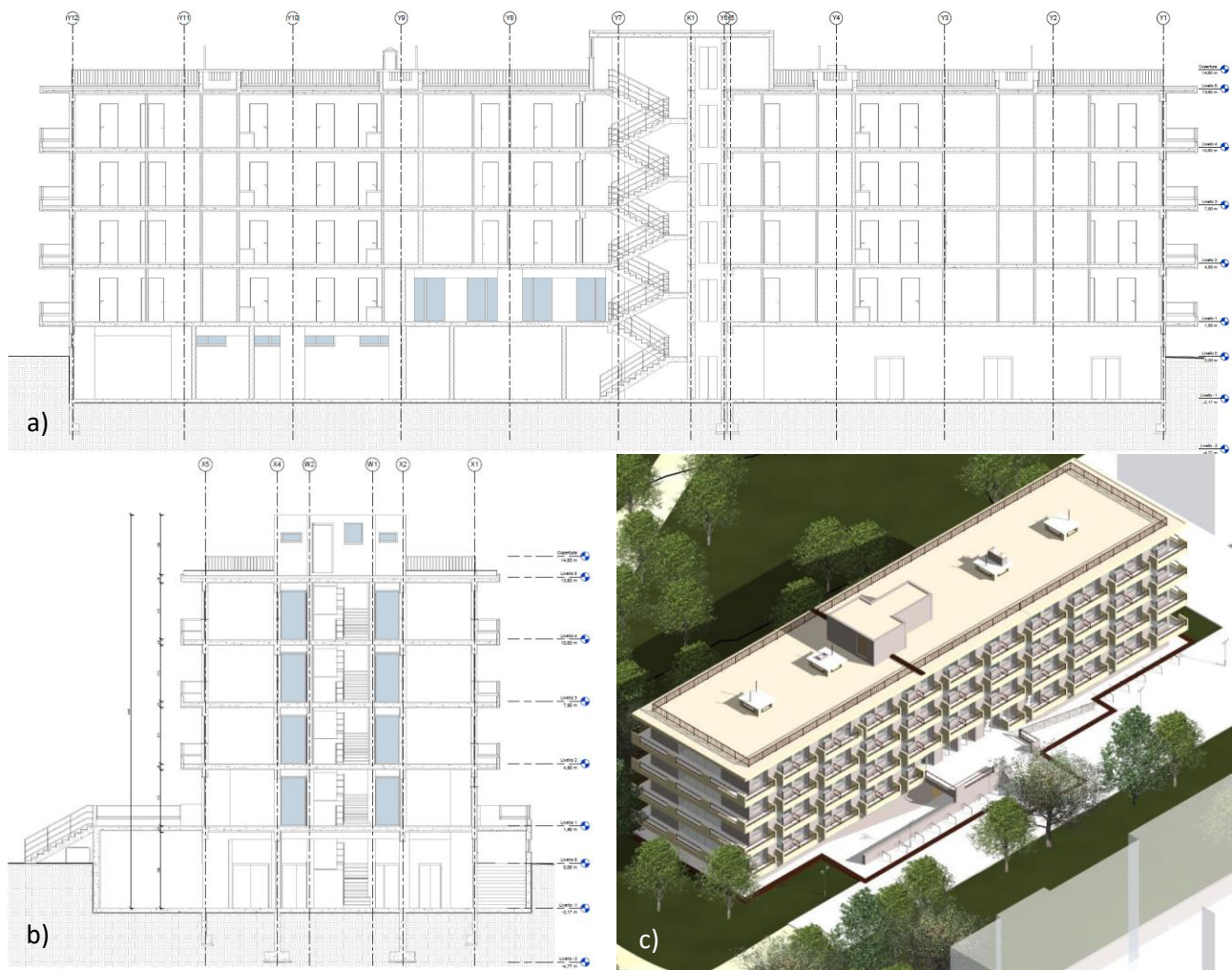
Figure 66 – Drawings of the initial state of the Athens case study; a) longitudinal cross-section; b) transversal cross-section; c) three-dimensional view of the BIM model – Source: [142]
