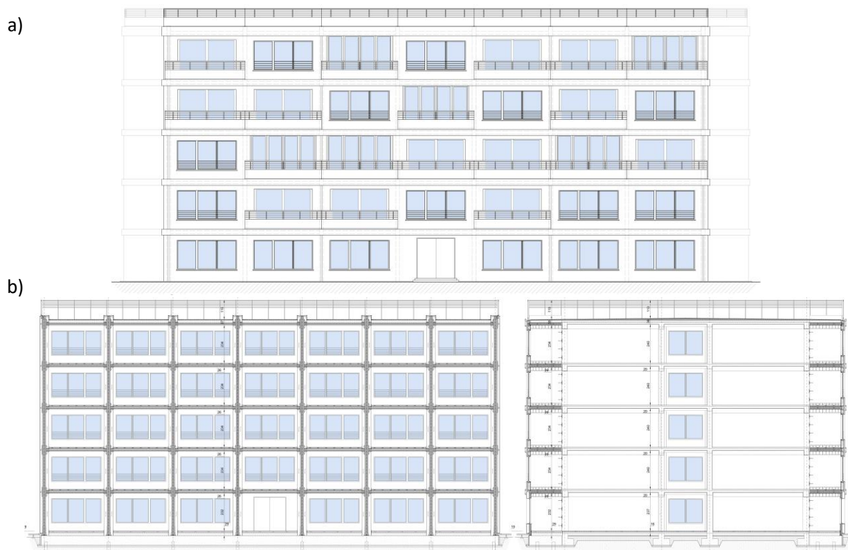
Figure 307 – a) Main façade of the project-state considering a randomised distribution of architectural units; b) vertical cross-sections of the project state considering the project-solution that provides only extra-room as architectural units of extension
