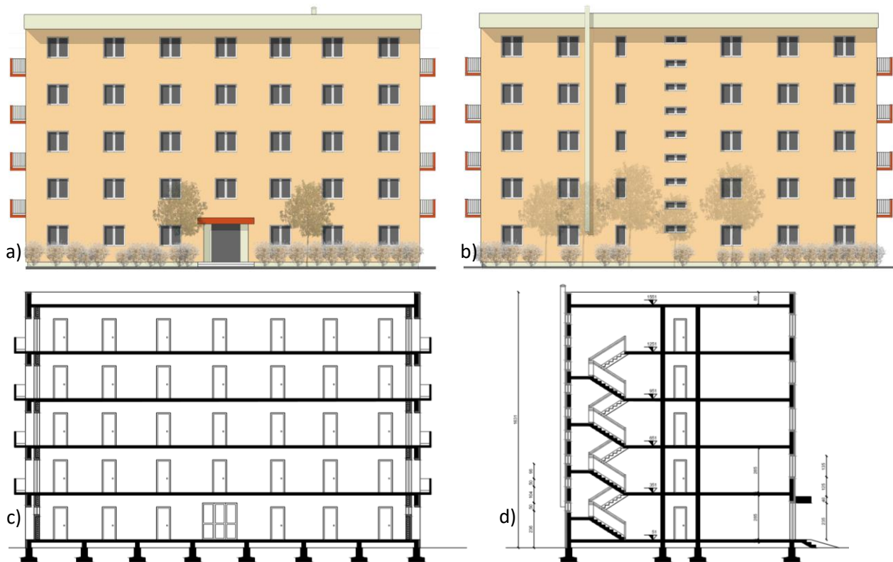
Figure 162 – Drawings of the initial state of the Brasov case study; a) north façade; b) south façade; c) longitudinal vertical cross-section; d) transverse vertical cross-section – Source: [159]
