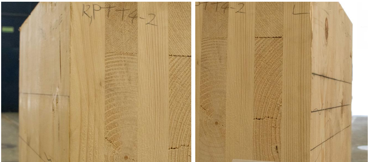
Figure 272 – Photos of the wall sample of PTT4-2 after the tests, showing no crushed grain on both the upper left and right sides
