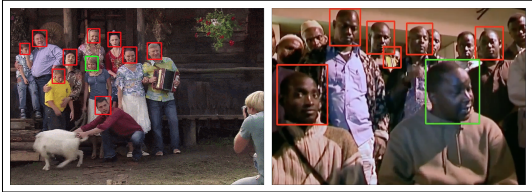
Figure 2.9: Examples from the AVA-ActiveSpeaker dataset [167]. Green and red bounding boxes imply speaking and not speaking classes, respectively.
