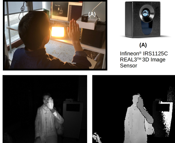
Figure A.1: Data collection setup. Dataset is collected in infrared (bottom-left) and depth (bottom-right) modalities using Infineon® IRS1125C REAL3™ 3D Image Sensor.
