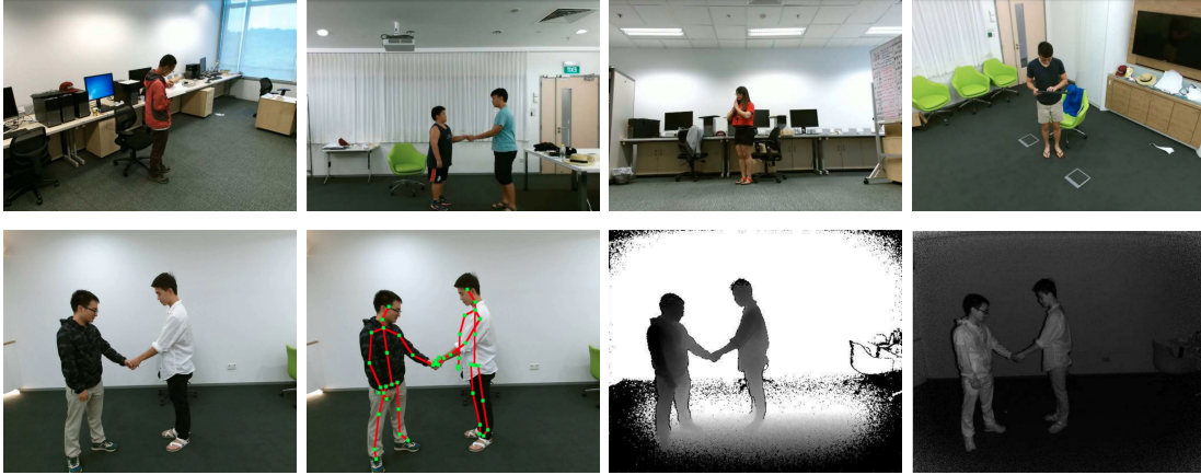
Figure 1.3: Example variations in video data. The top row illustrates variations in terms of human subjects and camera views. The bottom row illustrates variations in terms of video modality (from left to right: RGB, joint, depth, infrared). Examples are taken from the NTU RGB+D dataset [7].
