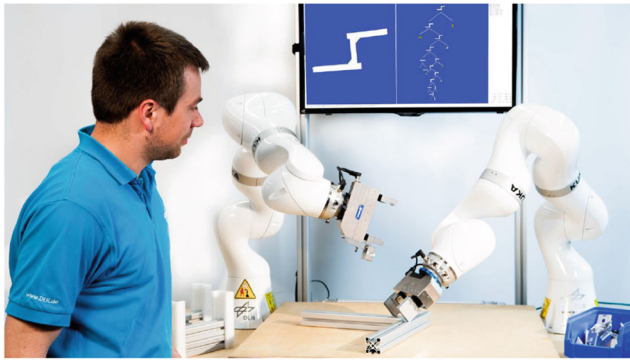
Fig. 1 Autonomous assembly of aluminum profile structures with a dual-arm robotic system without specialized holders
