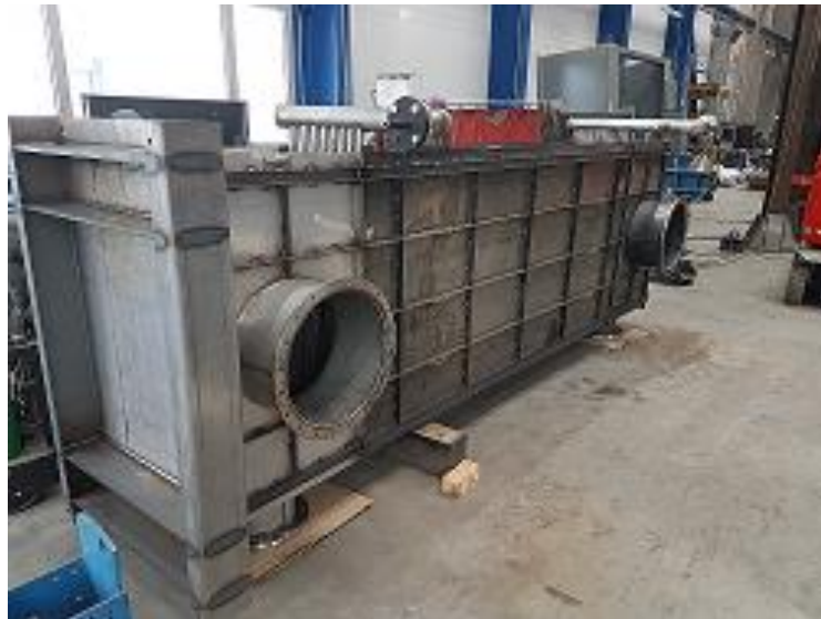
Figure 6: Water-tube-boiler prior to manufacturing quality control at APROVIS
