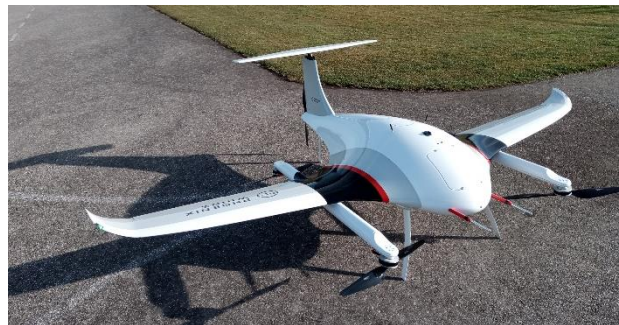
Figure 1: eVTOL UAV Manta Ray by Phoenix-Wings
