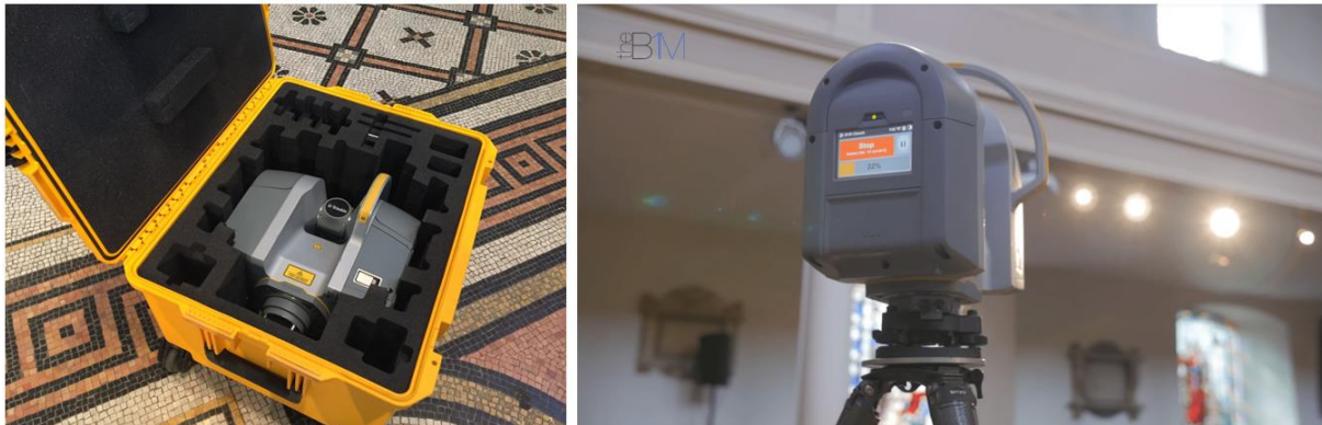
Figure 2: The Trimble TX8 in its portable case and on the tripod (B1M, 2017)
