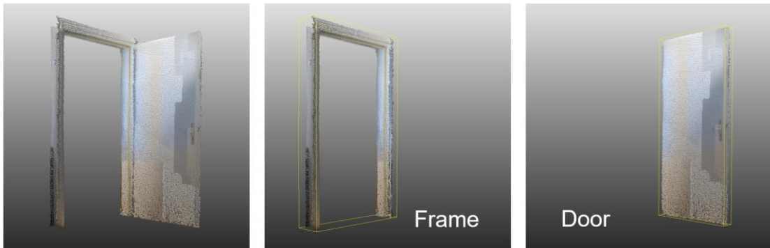
Figure 34: Segmentation of the object 'door' (Data Set I) into the objects 'door' and 'frame' (Data Set II)
