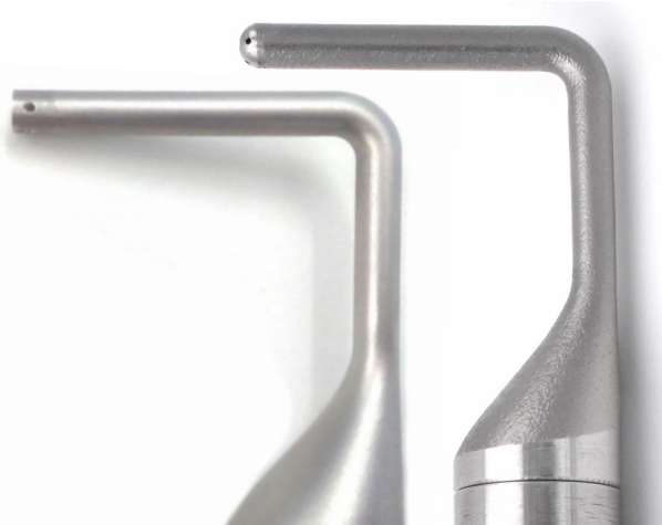
Figure 2.3: L-shaped probe head comparison: probe after additive manufacturing (left) and after post manufacturing process (right)
